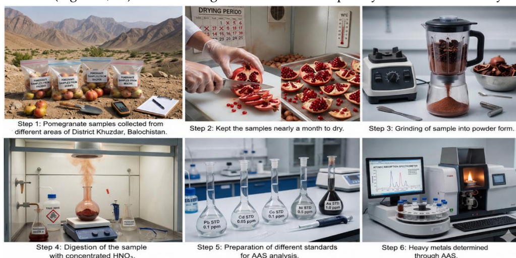
Fig. 1. Schematic representation of pomegranate sample preparation and heavy metal determination in pomegranate using Atomic Absorption Spectroscopy (AAS)
