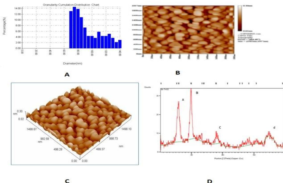
Fig. 1: X-ray diffractogram and AFM of Sb -TiO<sub>2</sub> (Anatase)
